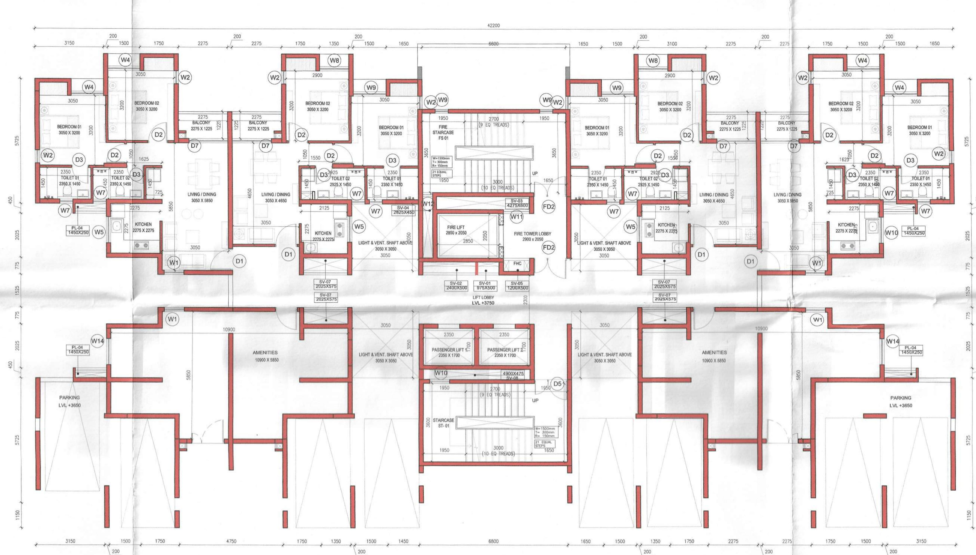
2 TOWER C2 PODIUM 01 FLOOR PLAN (LVL +3750) 1:100
